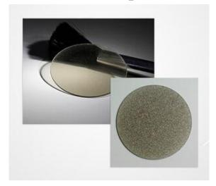
The good performance in broad-band optical transparency, high thermal conductivity and good hardness make diamond an ideal choice for highly demanding window applications such as high-power IR laser windows, high-power microwave windows and durable windows even in bad working conditions.
